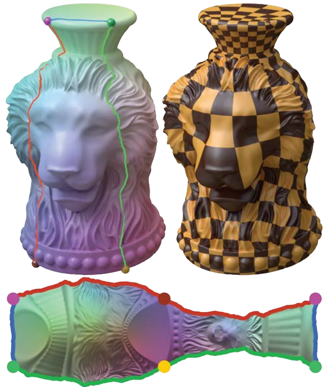
Figure 1: An example of the orbifold-Tutte embedding: a globally bijective mapping of a sphere-type surface (top-left) to a sphere-type Euclidean orbifold (bottom). In the orbifold, boundaries of the same color are topologically identified. Four points on the surface (shown as colored spheres, top-left) are mapped to the four cone singularities of the orbifold (colored disks, bottom). As in this case the orbifold has four cones, each of angle \pi , and they are placed on the integer grid, the embedding is also a quadrangulation, as shown on the top-right.
